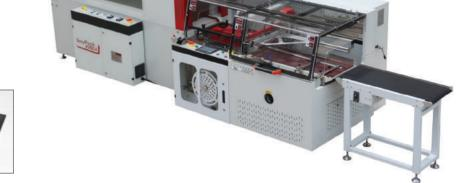
직선 Servo형 Sleeve Shrink Packing M/C
